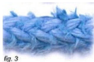
(Fig. 3) Severely braided rope
