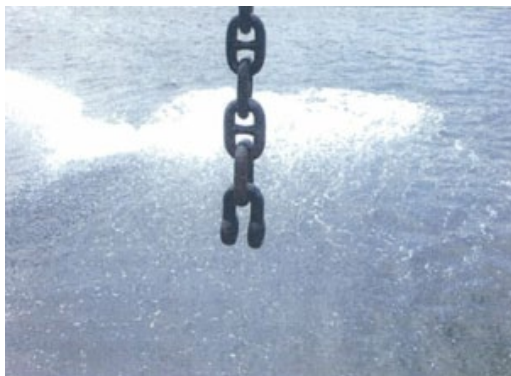
Pic.2 The anchor's joining shackle pin came off
