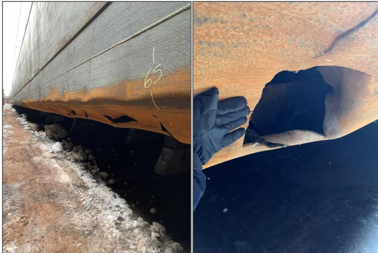
Figure 5. Damage to the port water ballast tanks.
